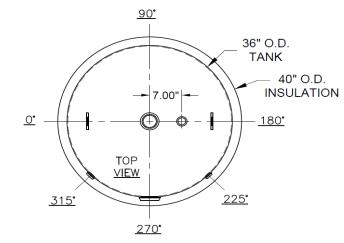
CONSTRUCTION: -MATERIAL - CARBON STEEL -INTERIOR LINING - PORCELAIN ENAMEL -EXTERIOR - PRIME PAINTED W/ 2" THK INSULATION & ACRYLIC TOP COAT -SACRIFICIAL ANODES - MAGNESIUM -M.A.W.P. - 125 PSI -MAX. OPERATING TEMP. - 180°F
