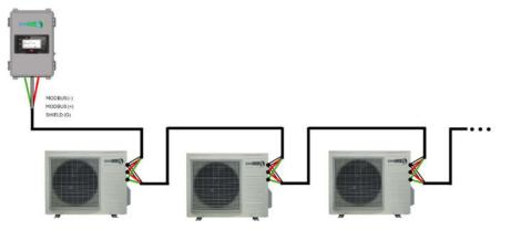
The network wiring must comply with Modbus RTURs-485 best practices, including:
