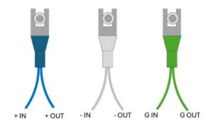
2. Connect a jumper wire (branch connection) to the HP's Modbus terminal. It is recommended to keep wires shorter than 3 ft.
