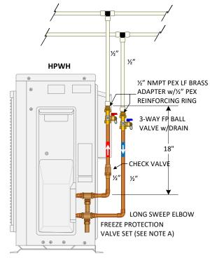
PIPING DETAIL B WITH PEX PIPE
