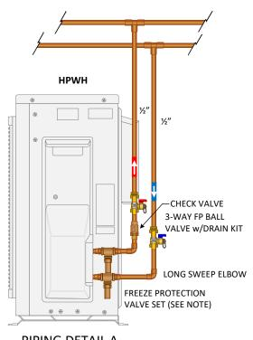
PIPING DETAIL A WITH COPPER PIPE
